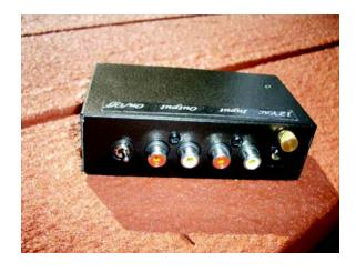
It's a real savior for those of us with middle-aged eyes. The front face is adorned by only the Vista Audio label. The back panel from left to right holds the POWER toggle switch, right and left input and output RCA jacks, brass ground wire connection screw and the socket for the outboard wall wort. The sides each hold two screws, and finally four rubber feet are attached to the base.
